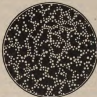
FIG. 15.—Appearance preceding coagulation in a concentrated gold solution. (According to H. Sidentopf.)
